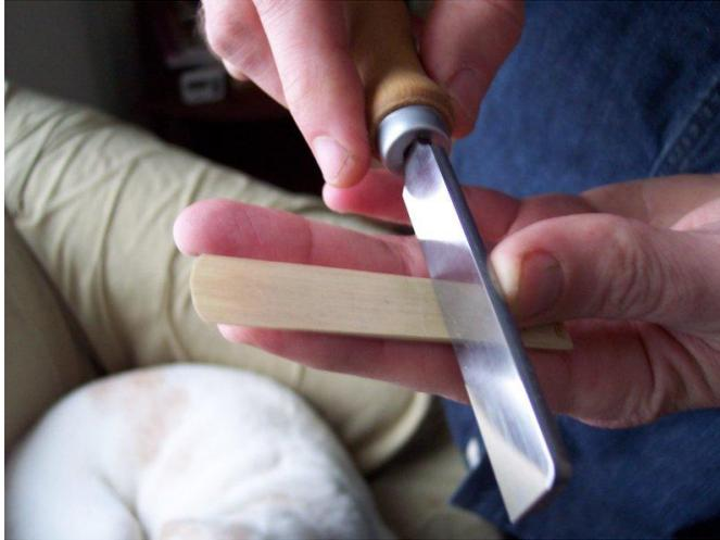
You want to flatten about the first two inches of the reed (tenor reed). The most important part is about half way up where the mouthpiece table ends and the mouthpiece window begins.
